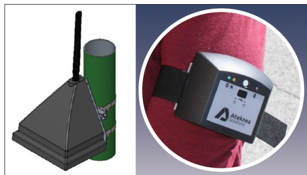
Static sensor pod by Geotech (left) and mobile sensor unit LEO (Little Environment Observatory; right), developed by ATEKNEA.
