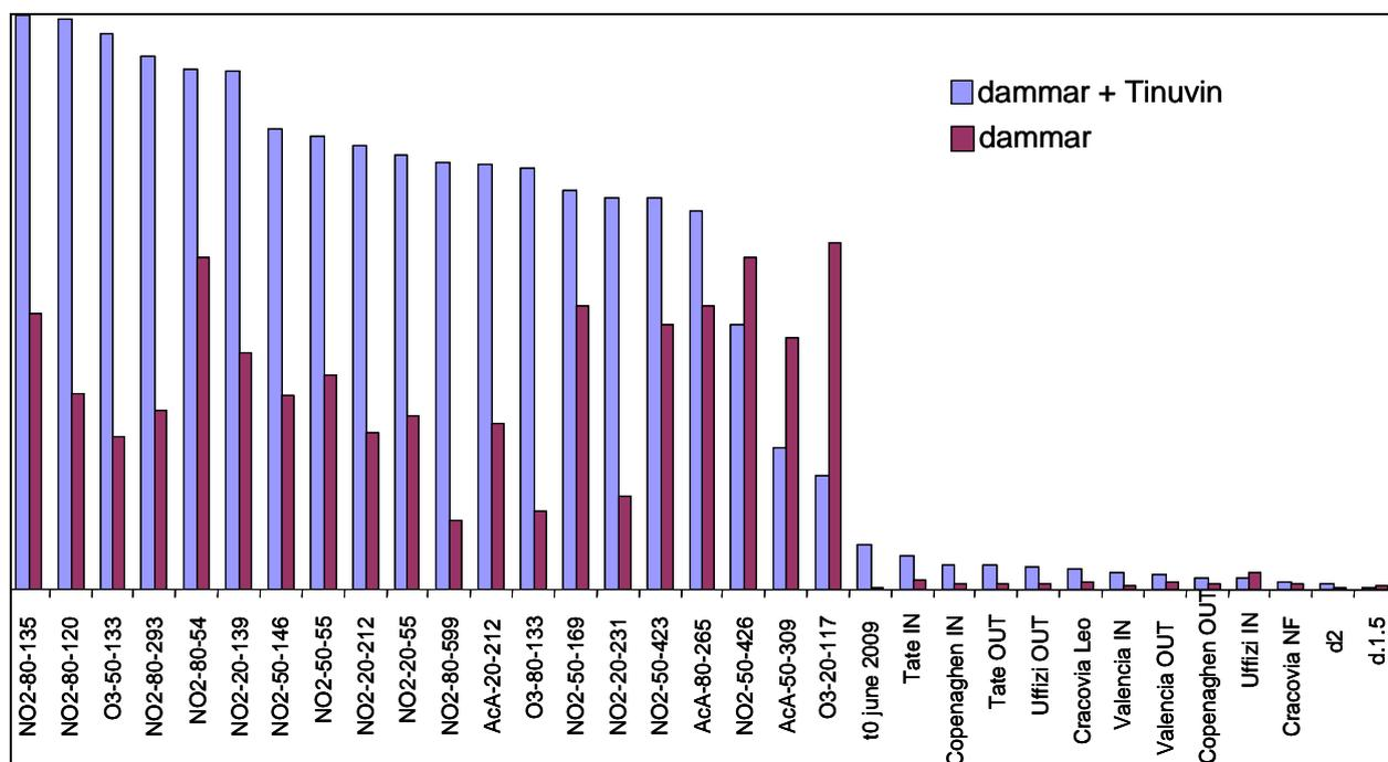
Figure 38: Amount of free triterpenoids in dammar resin after ageing, for the different ageing regimes (Table 10), with and without Tinuvin 292.
