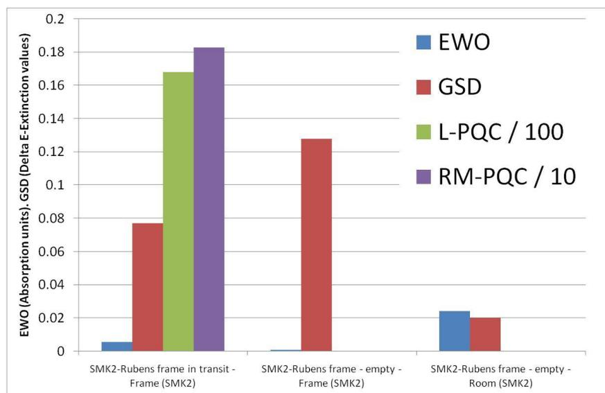
*Figure 15: Results from exposures of the EWO, GSD, L-PQCs and RM-PQCs inside and outside the SMK2 microclimate frame (Table 23). The units for the L-PQC and RM-PQC are % change and  $1000 \cdot f/F$  (= relation between the frequency shift and the original coated crystal frequency), respectively.*
