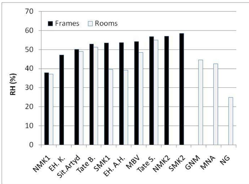
Figure 22: Mean relative humidity measured inside and outside the microclimate frames for paintings. For location abbreviations see Table 3 and table in Figure text 12.
