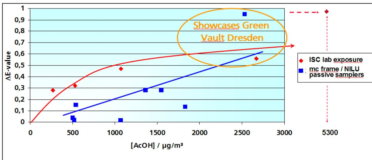
Figure 10: Environmental Glass Slide Dosimeters: correlation of  $\Delta E$ -values (3 months exposure) after acetic acid exposure vs. acetic acid concentration (all available data).
