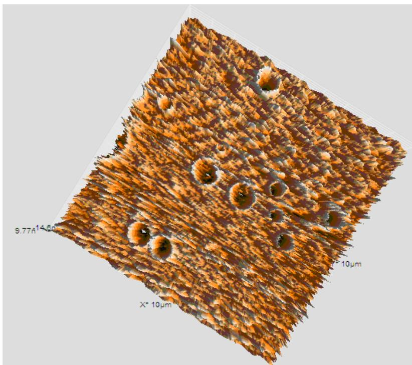
*Figure 53: AFM image (10 µm x 10 µm) of B72 exposed to NO<sub>2</sub> (4ppm for 27 days) at 80 % RH.*
