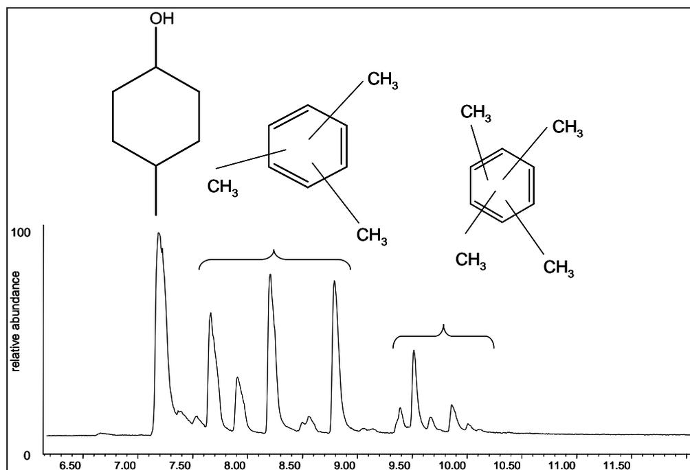
Figure 44: GC-MS chromatograms of MS2A resin of the varnish sample NO2-80-599 desorbed at 130°C.
