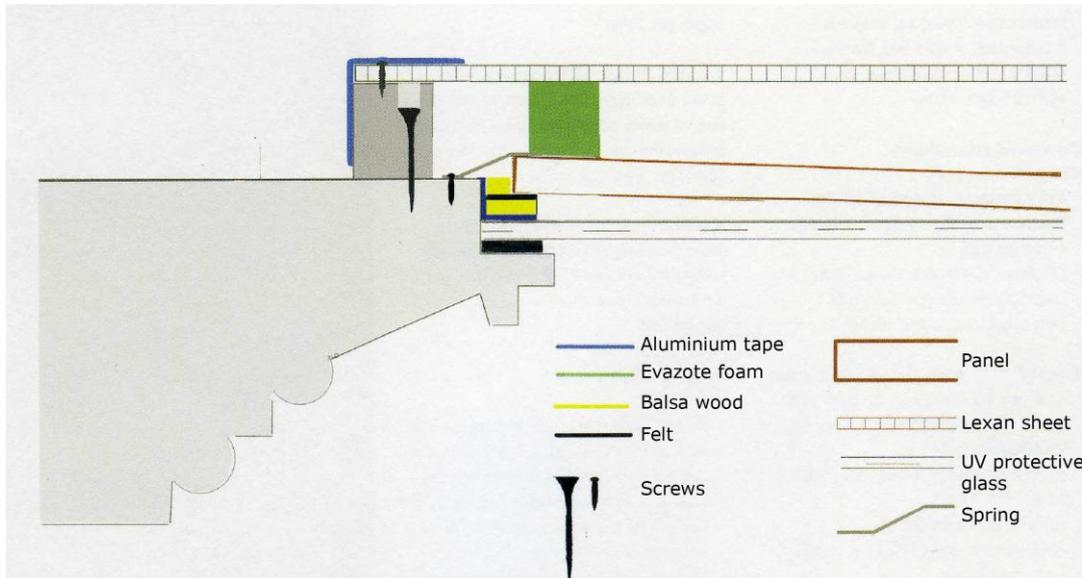
Fig. 1. Diagram showing cross-section of the construction of microclimate boxes used in the Mauritshuis.
