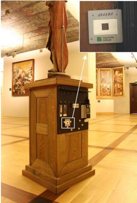
Figure 8: The Glass Slide Dosimeter developed by Fraunhofer ISC, exposed at the National Museum in Krakow, Poland.
