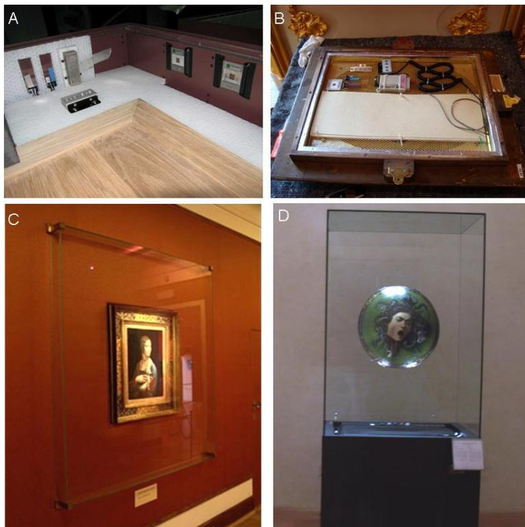
*Figure 11: Three dosimeters: 1. Early Warning Organic (EWO) dosimeter 2. Resin Mastic (RM-PQC) and Lead Piezoelectric Quartz Crystal (L-PQC) and 3. The Glass Slide Dosimeter (GSD), mounted inside the “modern” SIT-Artyd microclimate frame (A) and a “historic” frame adapted to microclimate frame at English Heritage, Apsley House, London, UK (B). C: Glass enclosure for painting (National Museum in Krakow). D: Showcase (Uffizi Gallery).*
