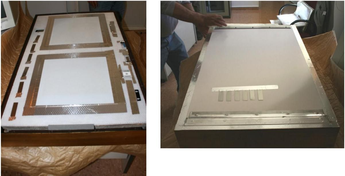
Figure 33: Museo de Bellas Artes de Valencia (ES). Inside (left) and outside (right) of the frame. The varnish samples were exposed in the darkness.
