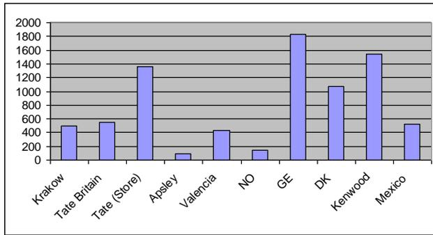
Figure 48: Acetic acid concentrations in frames.
