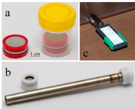
Figure 3: Examples of passive diffusion gas samplers for a) A range of gases depending on preparation of absorbing medium. b) Volatile Organic Compounds (VOCs) and c) Formaldehyde.
