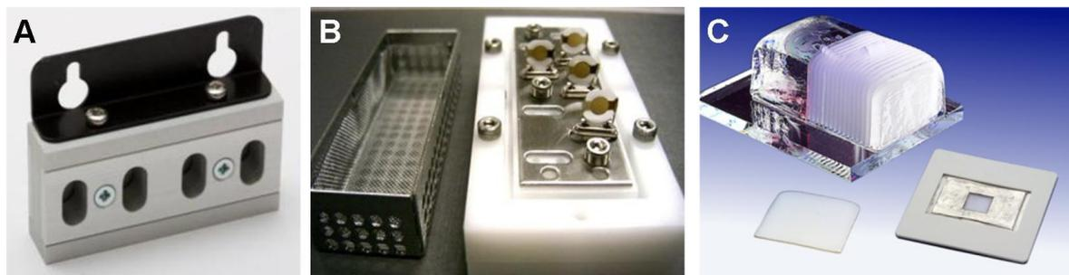
Figure 4: The main dosimeters used in the PROPAIN project: A. The NILU EWO (Early Warning dosimeter for Organic materials). B. The Birkbeck PQC (Piezoelectric Quartz Crystal) dosimeter and C. The Fraunhofer ISC GSD (Glass Slide Dosimeter).
