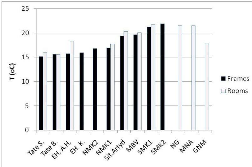
Figure 21: Mean temperature measured inside and outside the microclimate frames for paintings. For location abbreviations see Table 3 and table in Figure text 12.
