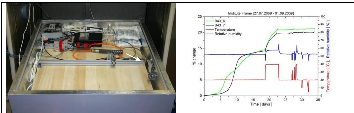
Figure 24: The position of the L-PQC dosimeter (crystals in flat silver holder) is shown using the arrow (left). The green and black traces show the change (%) in the crystals on exposure. The change occurs over the first 10/15 days. After 20 days the conditions in the microclimate chamber were changed (RH,T) (Right).
