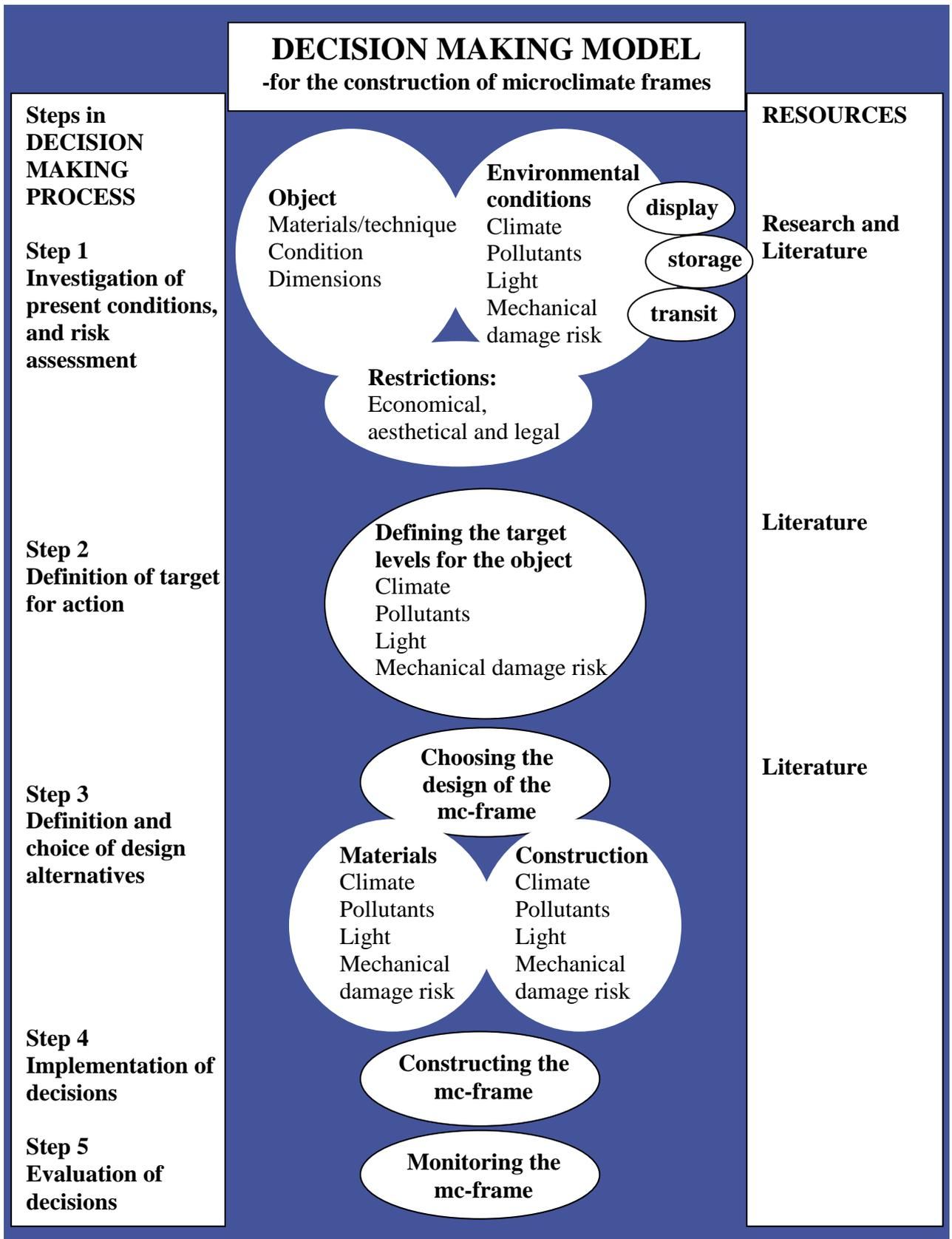
Figure 54: The PROPAIN Decision Making Model (mc-frame: microclimate frame).
