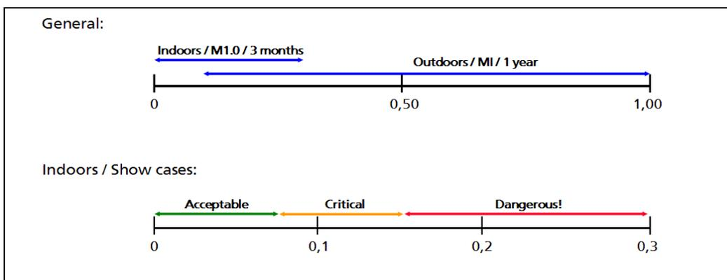
Figure 9: Environmental Glass Slide Dosimeters (type M1.0 and MI): range of exposure results ( $\Delta E$ -values) and related evaluation criteria after 3 month exposure (see also Figure 14).
