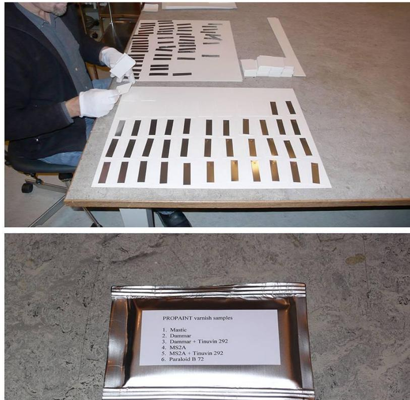
*Figure 29: Above: preparation of the varnish samples. Below: envelope containing a set of varnish samples.*
