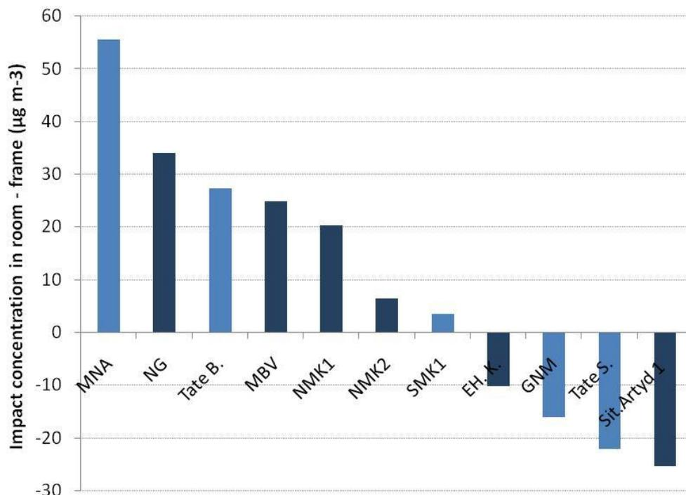
Figure 65: The protection effect against air pollutants of the microclimate frames at the end-user museums in PROPAIN, calculated as the “impact concentration” in the room minus the “impact concentration” still remaining inside the microclimate frame. (Dark blue bars are microclimate frames that were also modelled).
