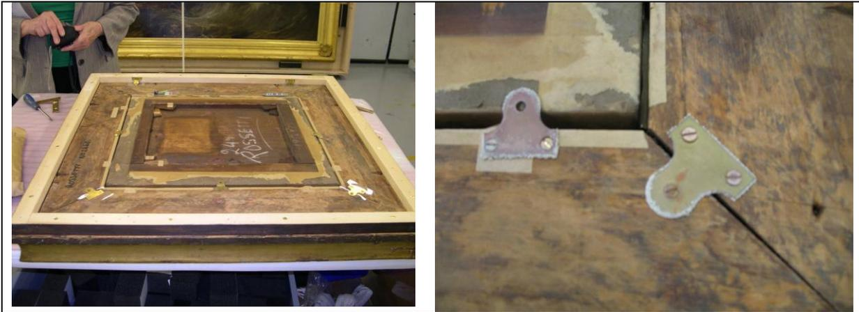
*Figure 26: Back of Rossetti painting with hardboard backing removed. Top right hand corner shows crystals mounted in steel frame and top left corner shows lead coupon and A-D strip (Left). Reverse of Rossetti painting showing deposits on brass plates (Right).*
