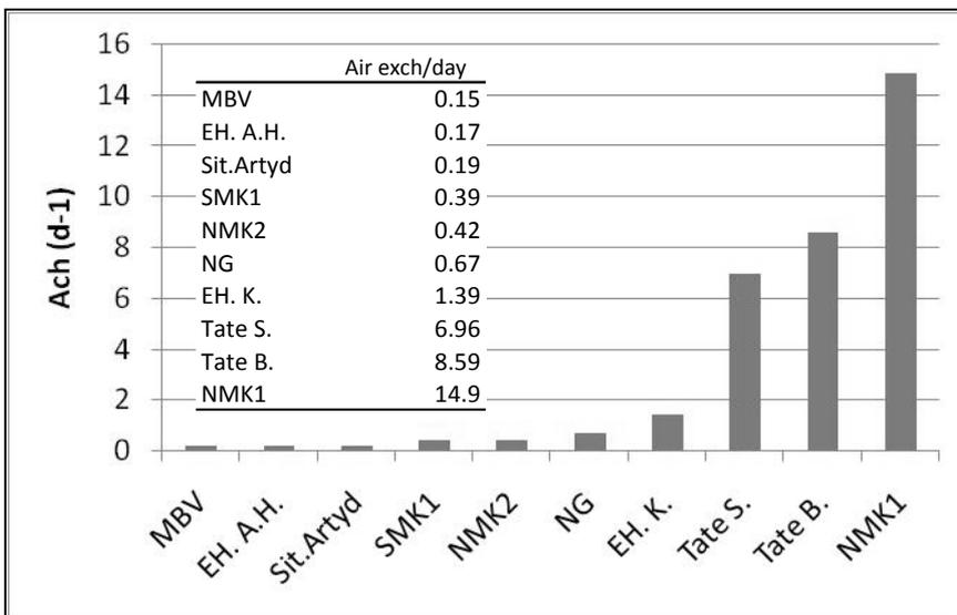
Figure 23: Air exchange rate of PROPAIN-microclimate frames. For location abbreviations see Table 3 and table in Figure text 12.
