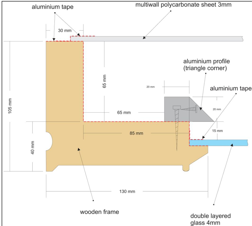
Figure 60: Microclimate frame for “epitaph of Jan Slupecki” (section).
