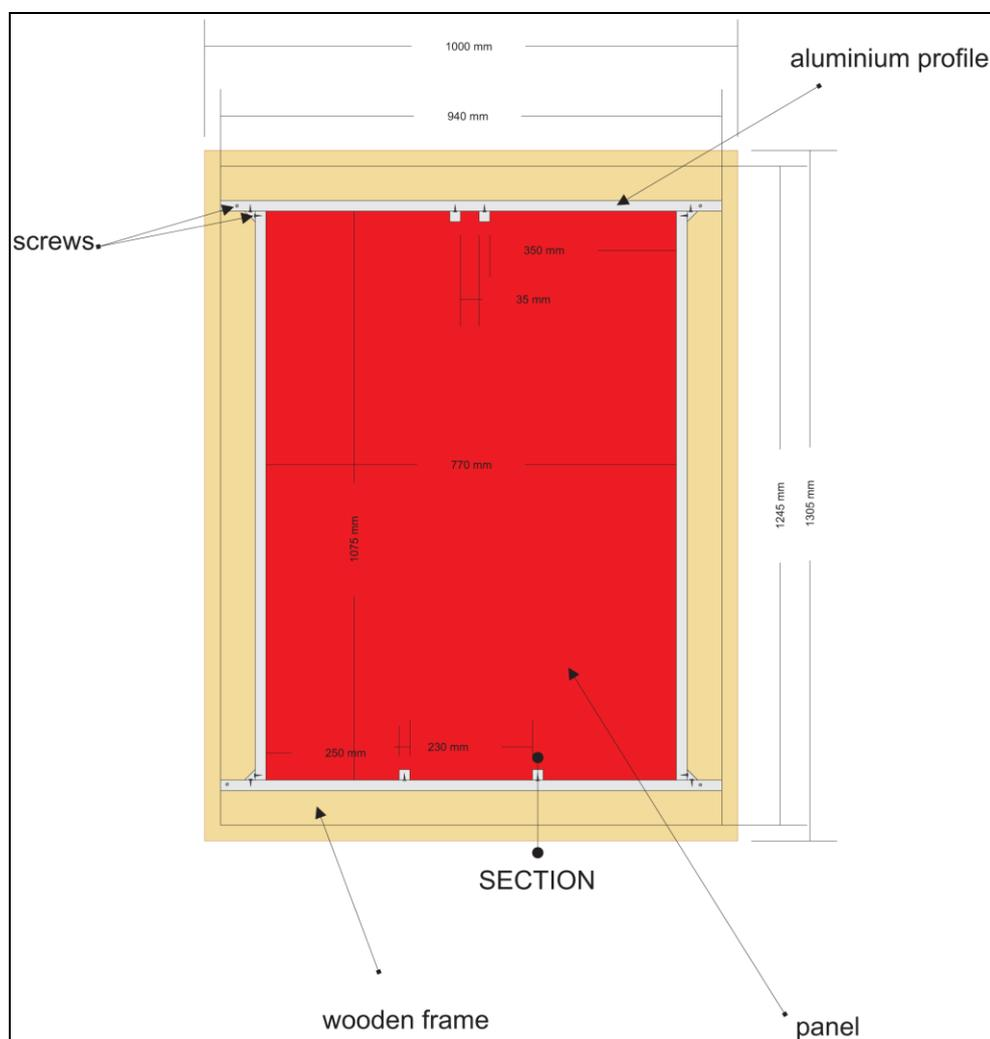
*Figure 59: Microclimate frame for “Epitaph of Jan Shupecki” (back).*
