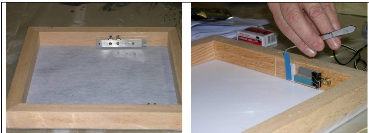
*Figure 25: Two lead coated PQC crystals were clamped in a steel support and fastened to one end of Frame no.2 containing Foamex (Left). Lead coupons and A-D strips were also mounted inside the frames (Right). Comparison was made between colour of unexposed strip held in tweezers and exposed strip for Frame no.2.*
